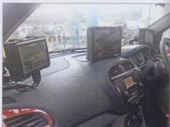
The surround view system, developed by Tata Ficoso, uses three screens, each providing a different visual.
