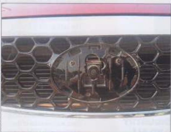
One of the wide-angle cameras mounted on the car exterior. Seen here is one of them mounted on the front grille.
