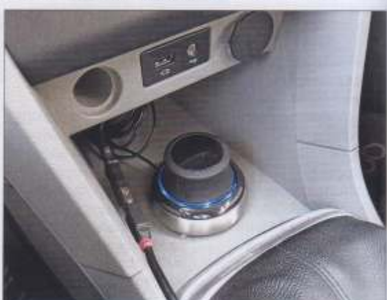
The joystick helps driver toggle between different visuals fetched by the four cameras mounted on each side of the car.
