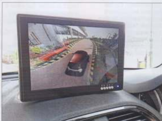
LCD screen mounted on the dashboard provides surround view including over-the-top visual of the vehicle (as seen).
