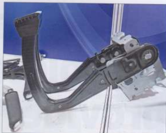
Another standout innovation is this aircraft-type parking brake lever for PVs, which offers space and aesthetic gains.
